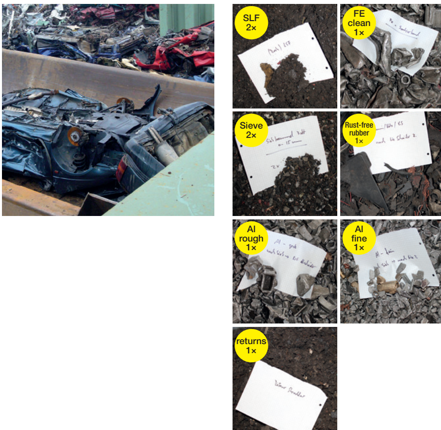
Diagram 5: Shredder input and samples from the output fractions
