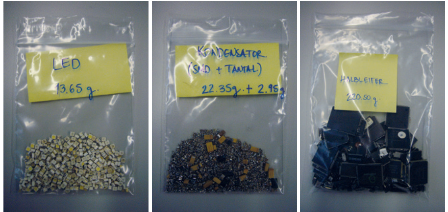
Diagram 4: Dismantled components and prepared samples from car electronic equipment
