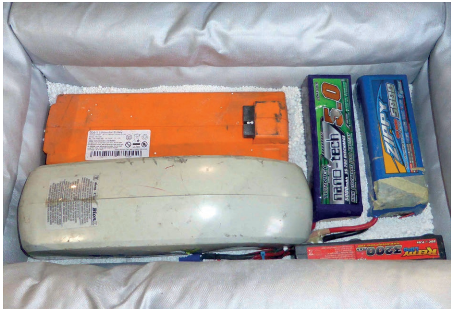
Figure 4: Fireproof box with a refractory lining material (PyroBubbles®) provided by Inobat for visibly damaged (swollen) or overheated lithium-ion batteries
