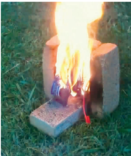
Figure 1: Burning lithium-ion battery
