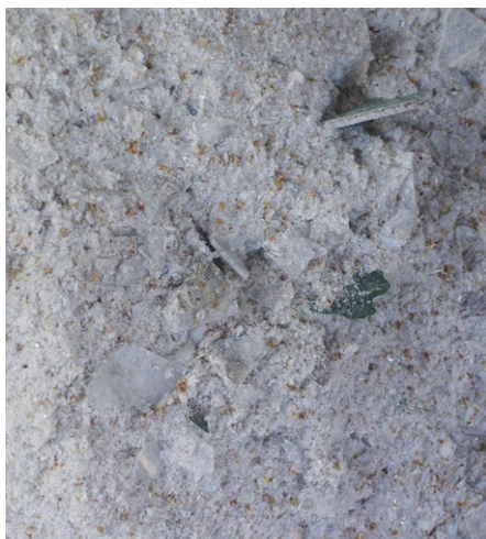
Figure 4: Luminescent-powder waste from gas-discharge lamps: a mixture of glass, mercury, rare earths and contaminants
