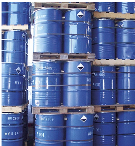
Figure 3: Drums filled with luminescent powder from a German lamp recycler ready for dumping underground (2010)
