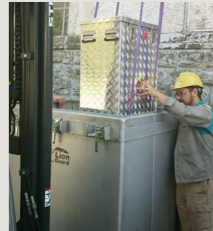
Figure 3: The UN-approved collection containers are lifted by harness into and out of the transportation containers.
