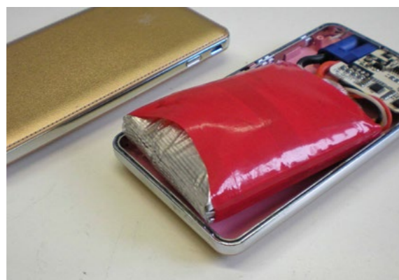
Figure 1: Clearly defective and dangerous LIB in notebooks or mobile phones. Such WEEE must be sorted out.
